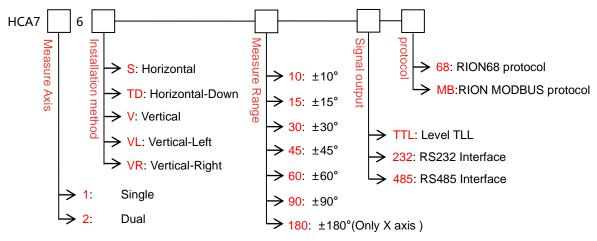
E.g : HCA716S-10-232-68 : Single axis / standard horizontal / ±10° measure range / RS232 signal output / RION68 protocol.
