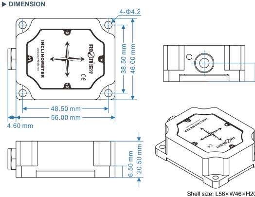
Shell size: L56×W46×H20.5mm Installation size: L48.5×W38×H6.5mm ounting screws: 4 M4 screws
